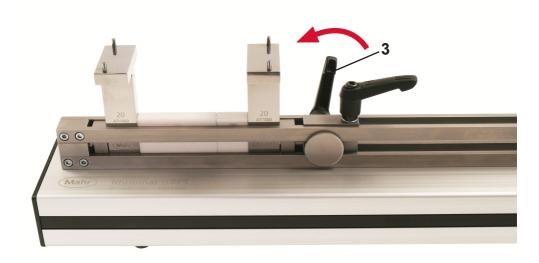
**7.4** Brace the parallel jaw/gage block combination securely by tightening the eccentric clamp using the tension lever **4**
