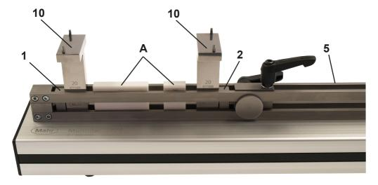
7.2 Put the tension lever for the eccentric clamp 4 in the middle position to pull back the mobile gage block clamping element
